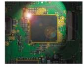
B channels. It also converts the signals to HD or SD format. With a performance equivalent to the processors used in many higher-end HD cameras, this DSP delivers beautiful images in all video formats.
